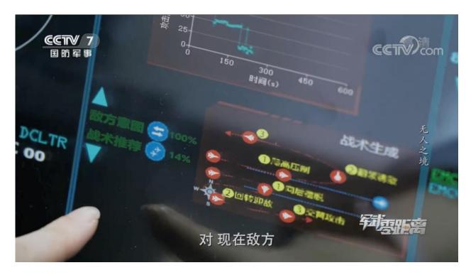
Figure 6: Image of CETC 28th Research Institute MUM-T loyal wingman simulator screen, displaying assessment of enemy intention, tactical recommendation, and several tactical maneuver options for the pilot<sup>104</sup>
